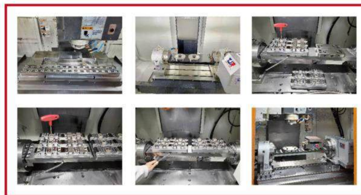
The illustration of the application for the zero point clamping system on the faceplate of the 4 th & 5 th axes
